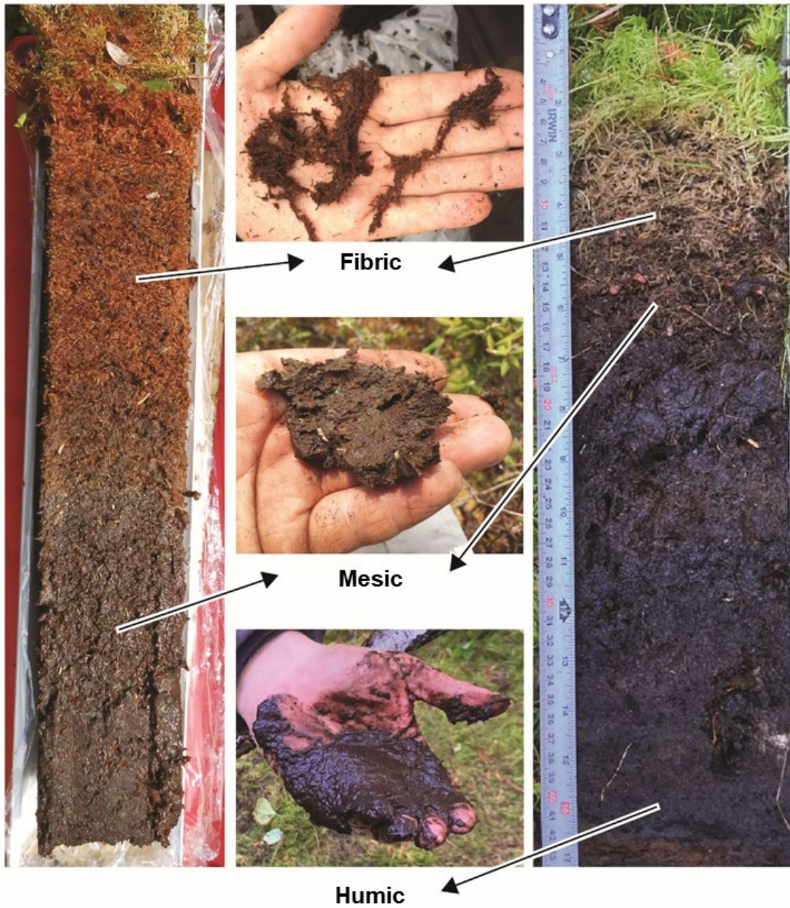
Figure 8. Degree of organic matter decomposition: fibric, mesic and humic. (See von Post scale in Appendix 1.)
