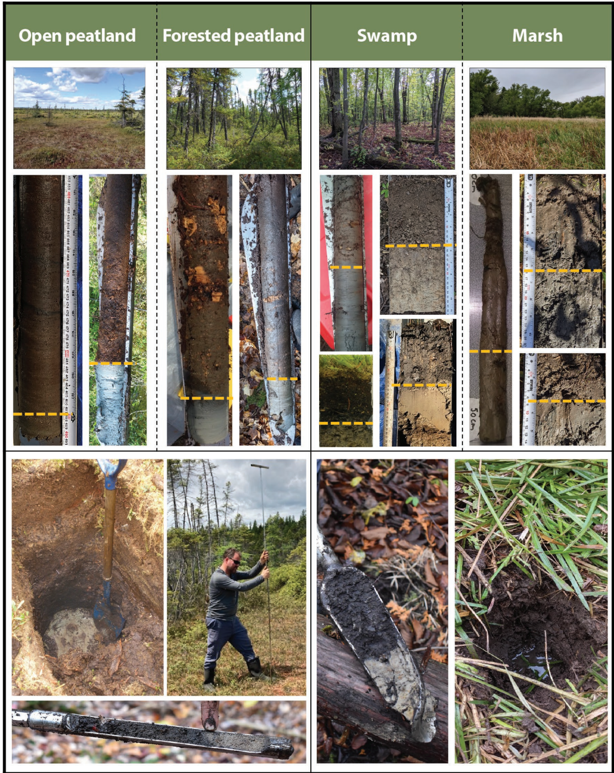
Figure 6. Measuring the thickness of organic deposits in different types of wetlands. The orange dashed lines represent the contact zone between the organic and mineral deposits.
