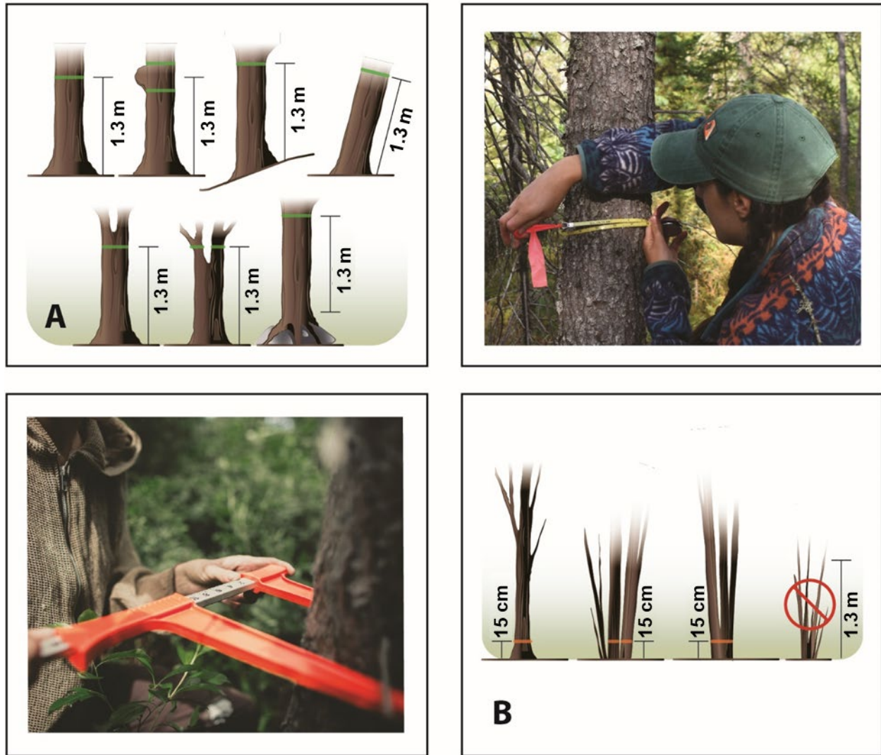
Figure 9. Location of the measurements of A) DBH and B) DSH according to different growth patterns for trees and shrubs.
