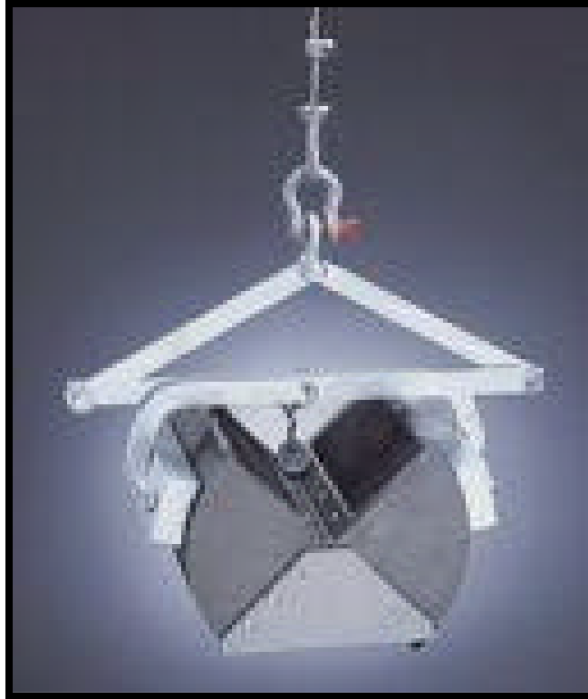
Figure 2: Ekman grab sampler attached to a winch for sediment sampling
