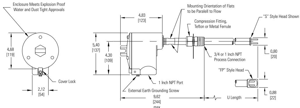
Enclosure: NEMA 4 Carbon Steel or NEMA 4X Aluminum
