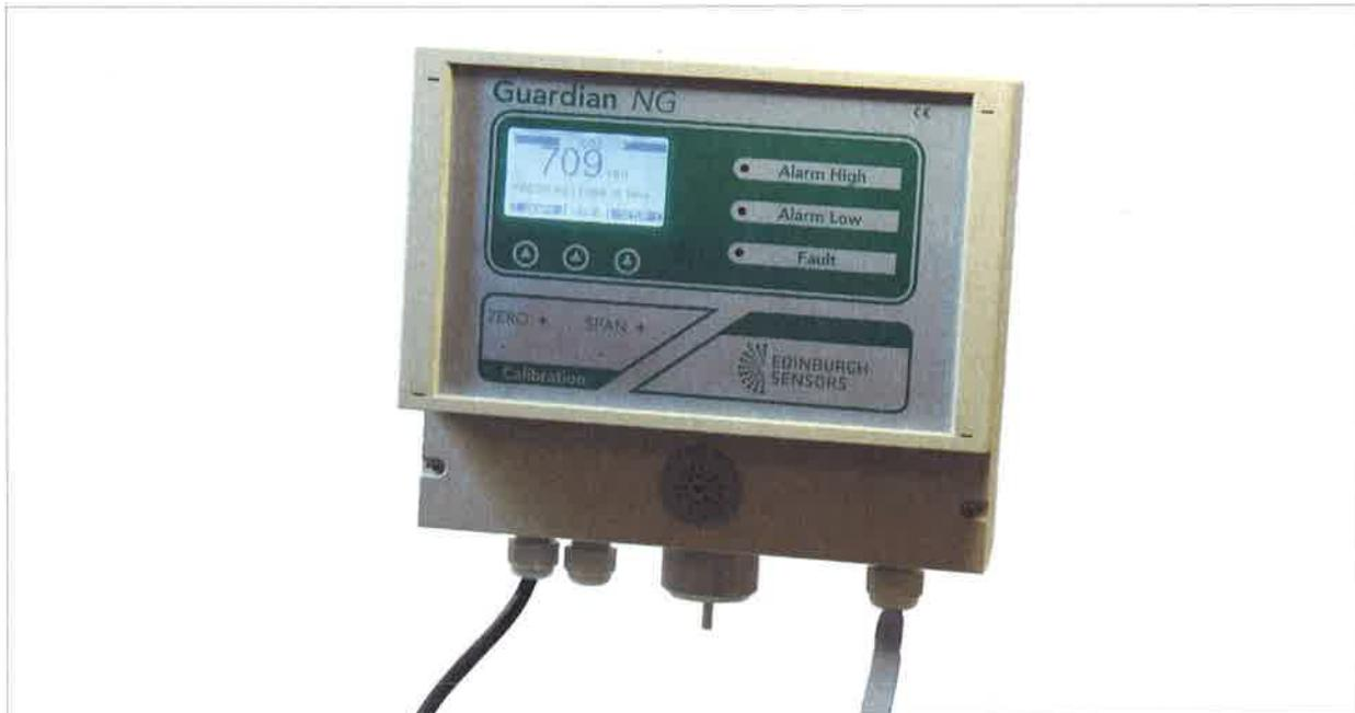
The NEW Guardian range of infrared gas monitors supplied by Edinburgh Sensors offers near-analyser quality, continuous sampling, measurement and display of target gas concentrations. The 'Guardian NG' range provides high accuracy detection and measurement of either CO<sub>2</sub> or CH<sub>4</sub> gases, where detection level ranges of between 0 – 3000ppm and 0 – 100% by volume are required.
