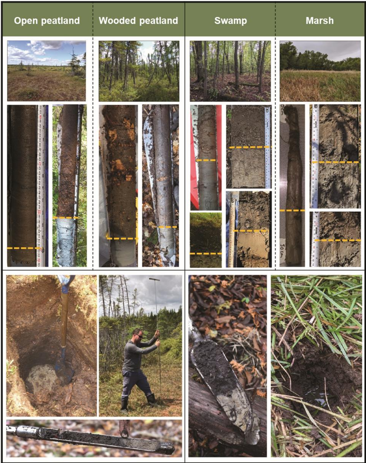
Figure 6. Measuring the thickness of an organic deposit in different types of wetlands. The orange dashed lines represent the contact zone between the organic deposit and the mineral deposit.
